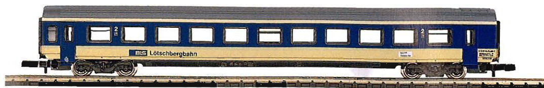
V 87461 Express Train Passenger Car. Mark IV type B coach. 2nd class. Length over buffers 120 mm (4-3/4").
