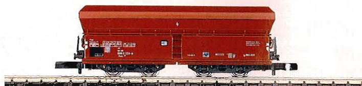
IV 8630 Hopper Car. Type Fals 176. Length over buffers 53 mm (2-1/8").
