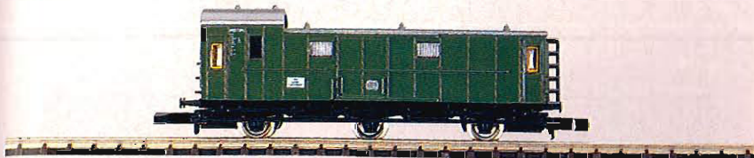
III 8703 Baggage Car. Former type Pw3-pr02. Length over buffers 57 mm (2-1/4").
