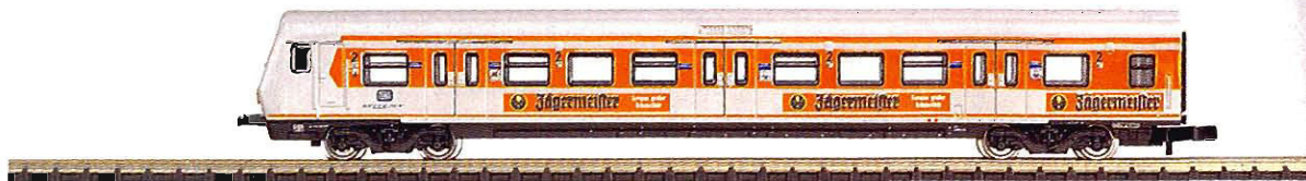
V 87980 S-Bahn Car. Type ABx 791.1 with advertising along the car's sides for "Bauknecht". 1st and 2nd class. Length over buffers 111 mm (4-3/8").
