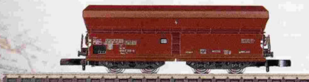
IV 8630 Hopper Car. German Federal Railroad (DB) type Fals 176. Length over buffers 53 mm (2-1/8").
