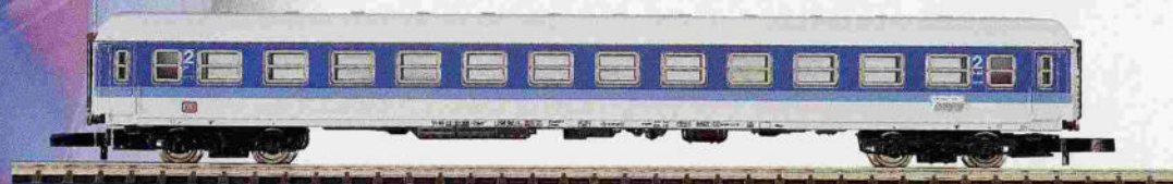
V 8744 InterRegio Coach. German Federal Railroad (DB) type Bim, in the current color scheme. 2nd class. Length over buffers 120 mm (4-3/4").
