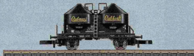
III 86661 Silo Container Car. Type Ucs 909. Privately owned by Club-Kraftfutterwerke GmbH, Mannheim, Germany. Used on the German Federal Railroad (DB). Length over buffers 40 mm (1-9/16").
