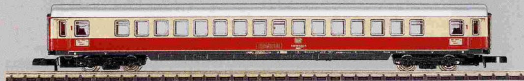
IV 8725 TEE/IC Open Seating Coach. German Federal Railroad (DB) type Apmz. 1st class. Length over buffers 120 mm (4-3/4").
