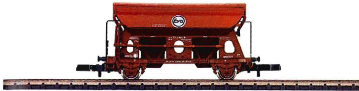
V 82375 Side Dump Car with Hinged Roof. Prototype: Type Td. Car privately owned by Eva, Railroad Transport Services, Inc., Düsseldorf, Germany. Used on the German Railroad, Inc. (DB AG). Model: Hinged roof that can be opened. Separately applied railings, ladders, and hatch levers. Length over buffers 43 mm / 1-11/16".
