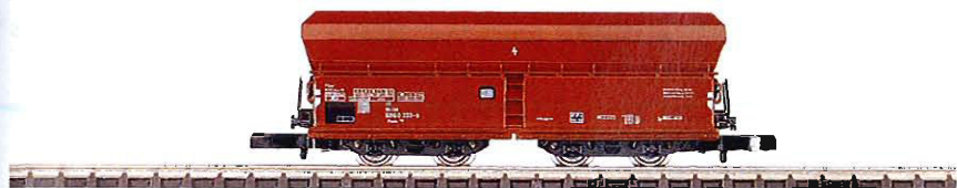
IV 8630 Hopper Car. Prototype: German Federal Railroad (DB) type Fals 176. Model: Length over buffers 53 mm / 2-1/8".
