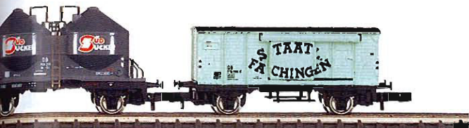
IV 8624 Ballast Car. Prototype: Talbot self-dumping car for maintenance work on the German Federal Railroad (DB). Model: Unloading hatches that can be opened. Length over buffers 33 mm / 1-5/16".
