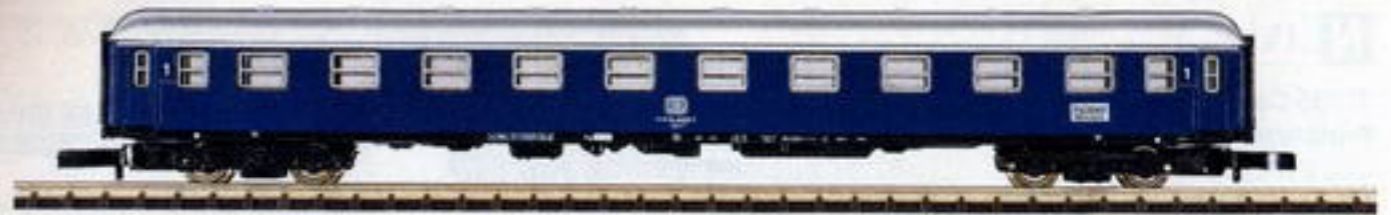
IV 8710 Express Train Passenger Car. Prototype: German Federal Railroad (DB) type Am 203. 1st class. Model: Length over buffers 120 mm / 4-3/4".
