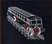
Track-cleaning railcar · 2 driven axles · Automatic coupling at car end · Length over buffers 62 mm (2-7/16")
