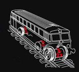
Track-cleaning car · 2 powered axles · Automatic coupler on rear end · Length over buffers 62 mm (2-7/16")
