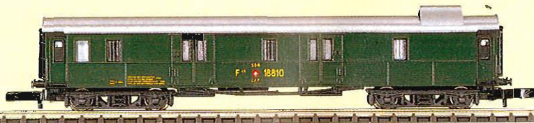
8748 Express Train Passenger Car. Older design C4ü. 3rd class. Length over buffers 87 mm (3-7/16").
