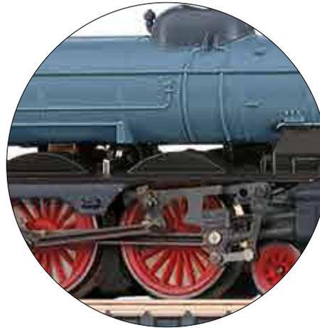
Finely detailed valve gear
